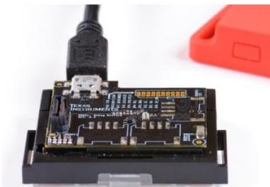
**Figure 4. CC1350STK with attached DevPack board**
