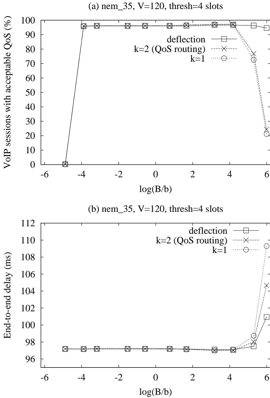
Figure 12: Results for an irregular topology with 35 nodes: (a) fraction of VoIP channels with acceptable QoS and (b) end-to-end delay
