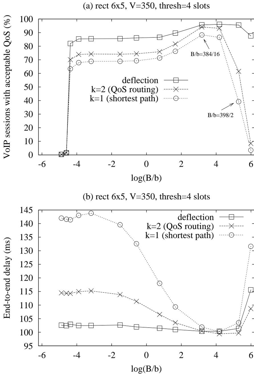
Figure 5: Rectangular topology with 350 simultaneous VoIP sessions and threshold set to 4 slots: (a) fraction of VoIP sessions with acceptable QoS and (b) end-to-end delay
