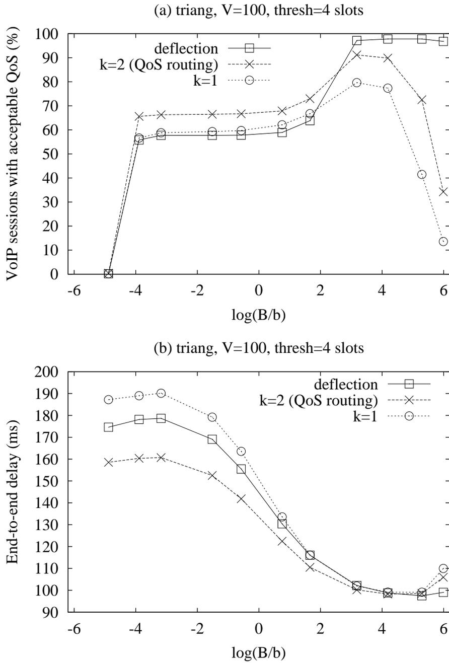
Figure 10: Results for triangular topology: (a) fraction of VoIP channels with acceptable QoS and (b) end-to-end delay
