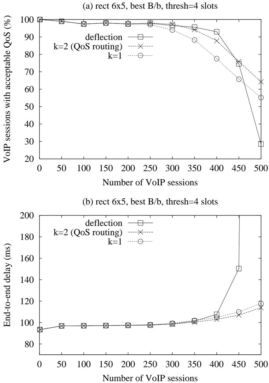
Figure 6: Rectangular topology with threshold set to 4 slots: (a) fraction of VoIP sessions with acceptable QoS and (b) end-to-end delay
