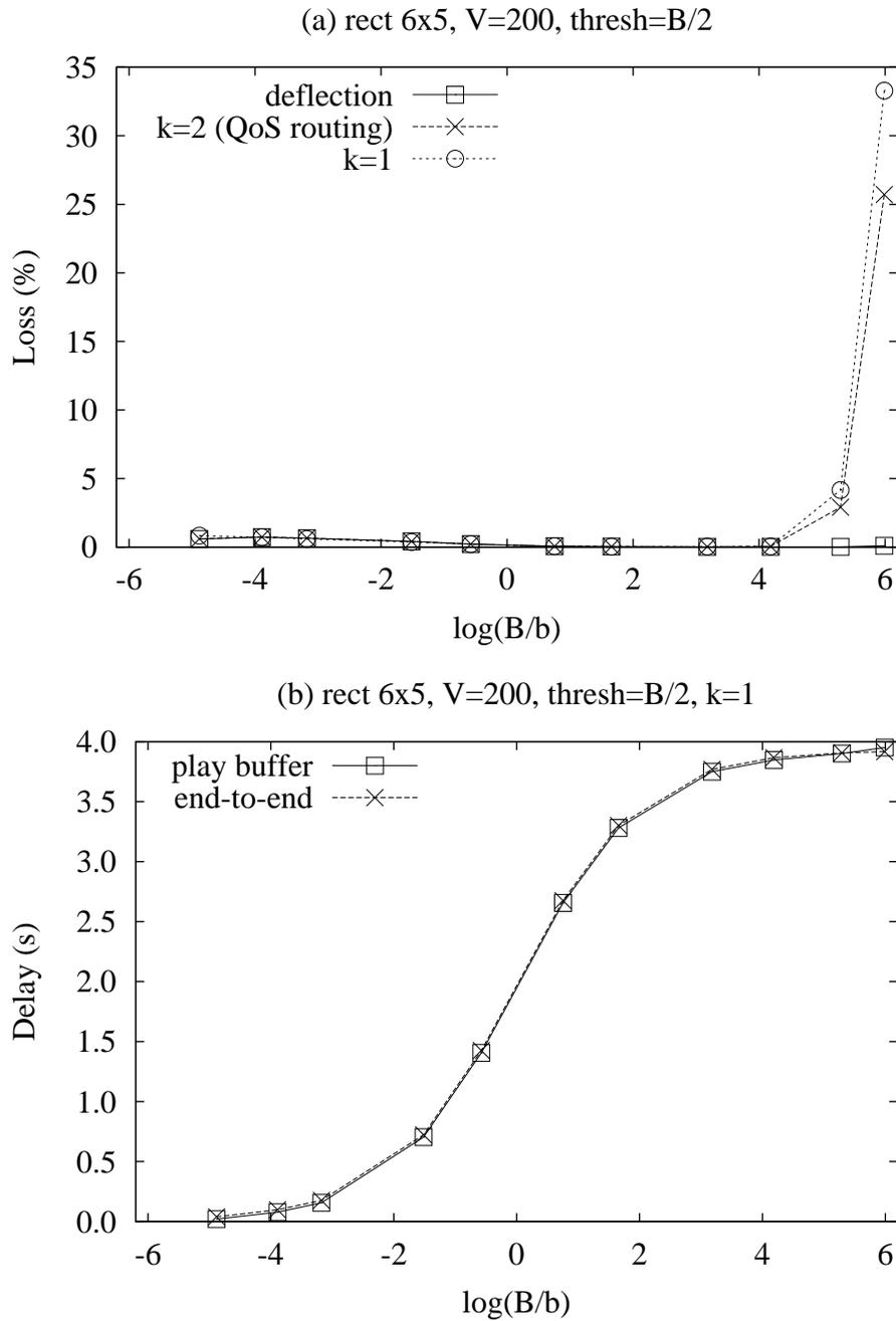
Figure 3: Rectangular topology with threshold equal to half the reassembly buffer size: (a) loss rate and (b) delay
