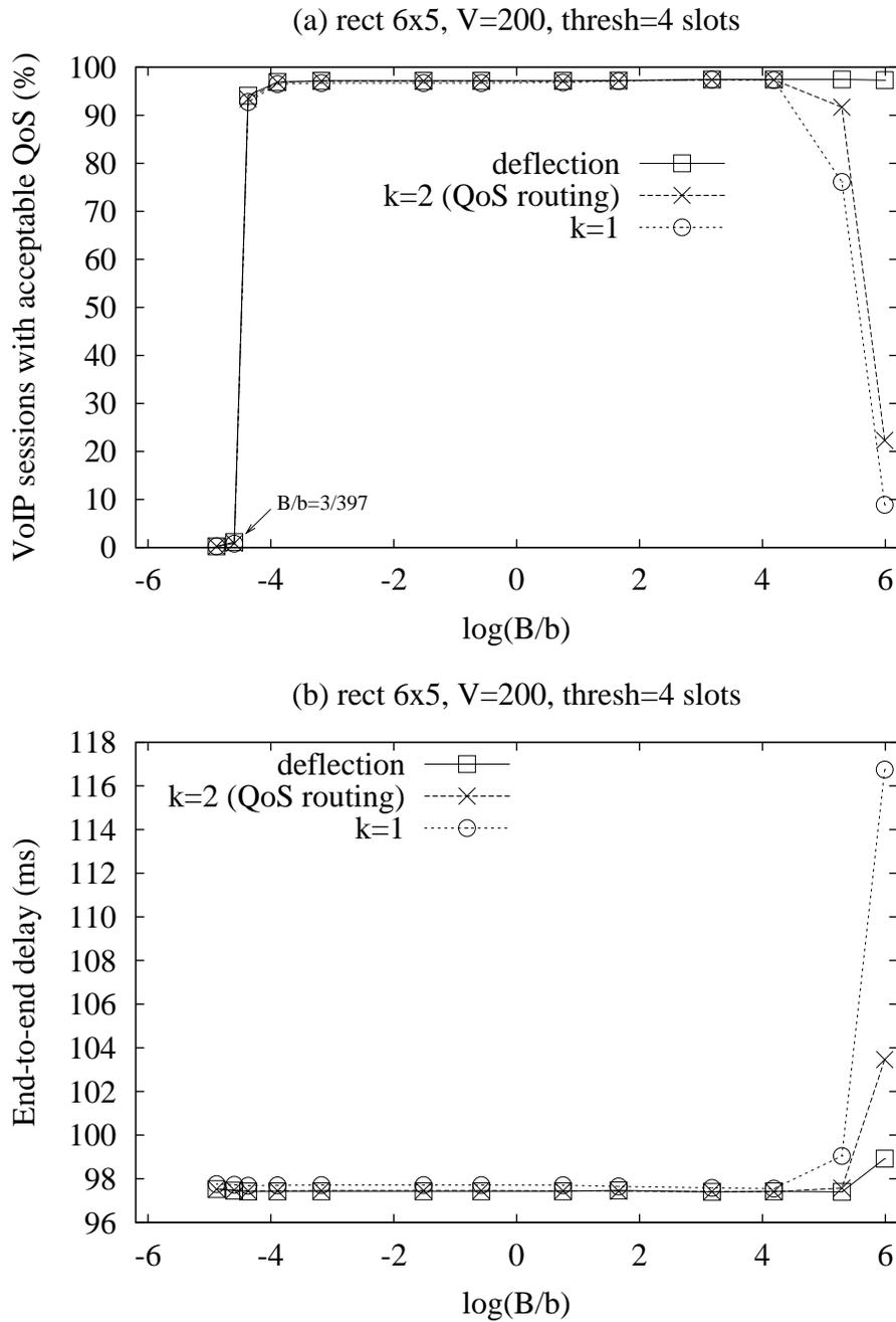
Figure 4: Rectangular topology with 200 simultaneous VoIP sessions and threshold set to 4 slots: (a) fraction of VoIP sessions with acceptable QoS and (b) end-to-end delay
