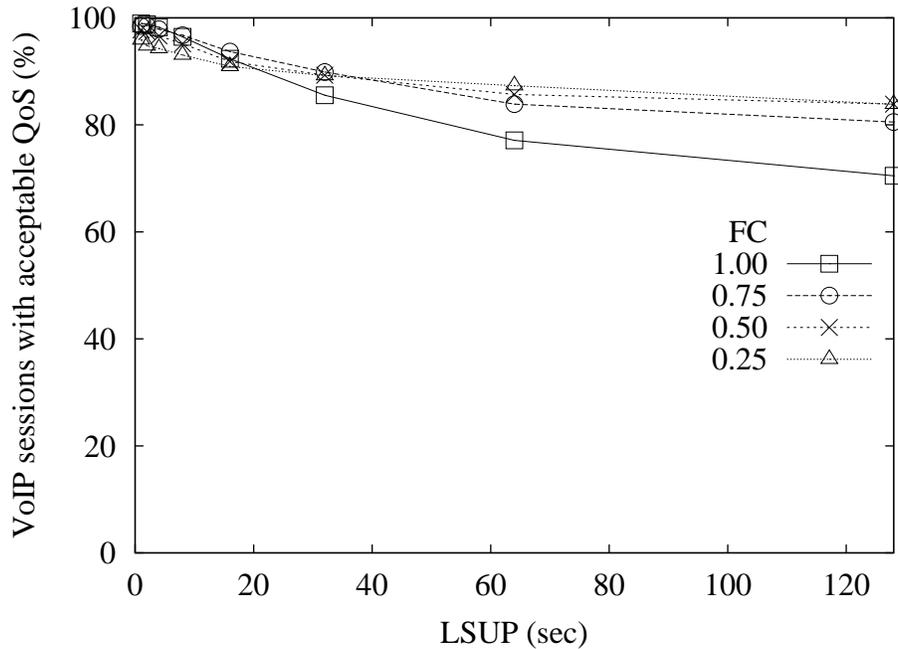
Figure 8: Fraction of VoIP sessions with acceptable QoS versus LSUP for different Frequency Coefficients (FC) on the rectangular topology
