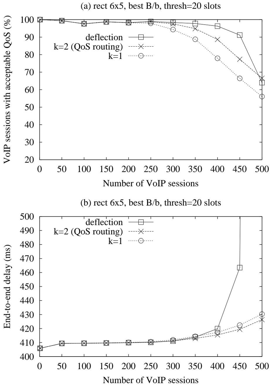
Figure 7: Rectangular topology with threshold set to 20 slots: (a) fraction of VoIP sessions with acceptable QoS and (b) end-to-end delay
