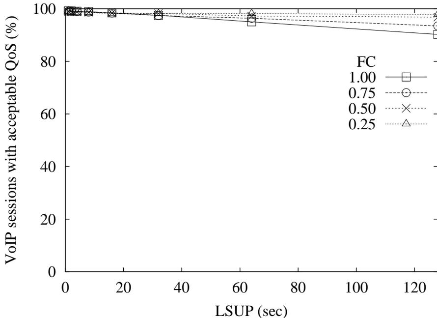
Figure 11: Fraction of VoIP sessions with acceptable QoS versus LSUP for different Frequency Coefficients (FC) on the triangular topology
