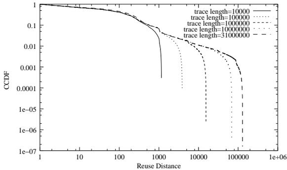
**Fig. 2** Measured reuse distance CCDF's
