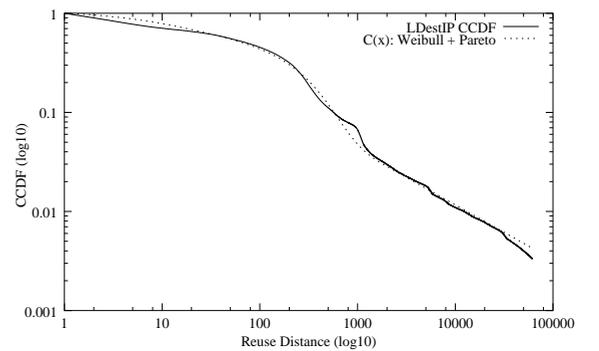
**Fig. 3** Fitting a reuse distance CCDF with Eq. 8
