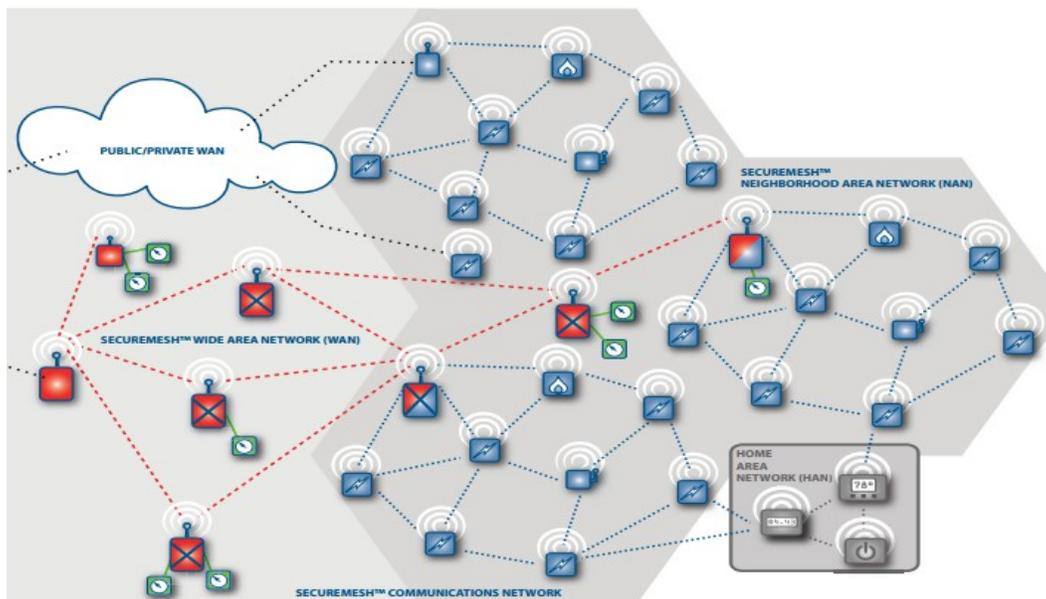
Abstracted from many necessary and attractive features, the system senses, collects and delivers meter readings interactively and/or for off-line processing. Whenever any of the nodes/meters forward information in an ad-hoc manner, we enter the main area of our presentation.
